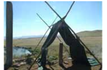
Measurement setup with a tent to avoid sunlight interference
